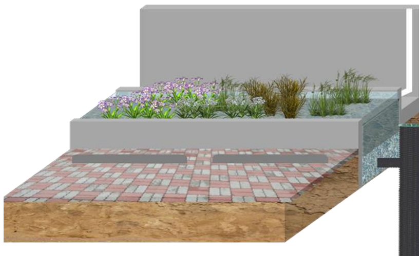
Flow-Through Planter Box with Typical Features
